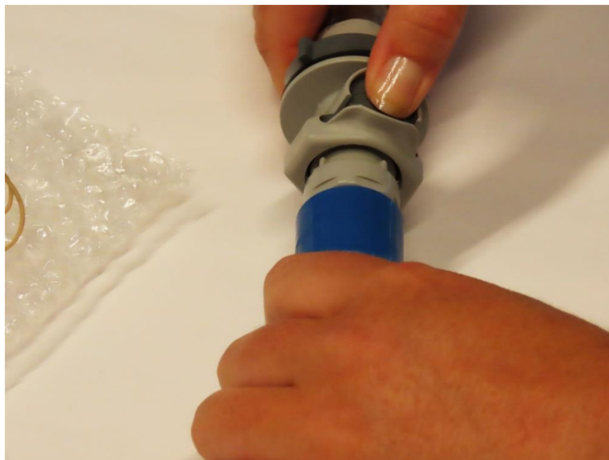
Figure 17. Inserting the process connector into the bag connector.
