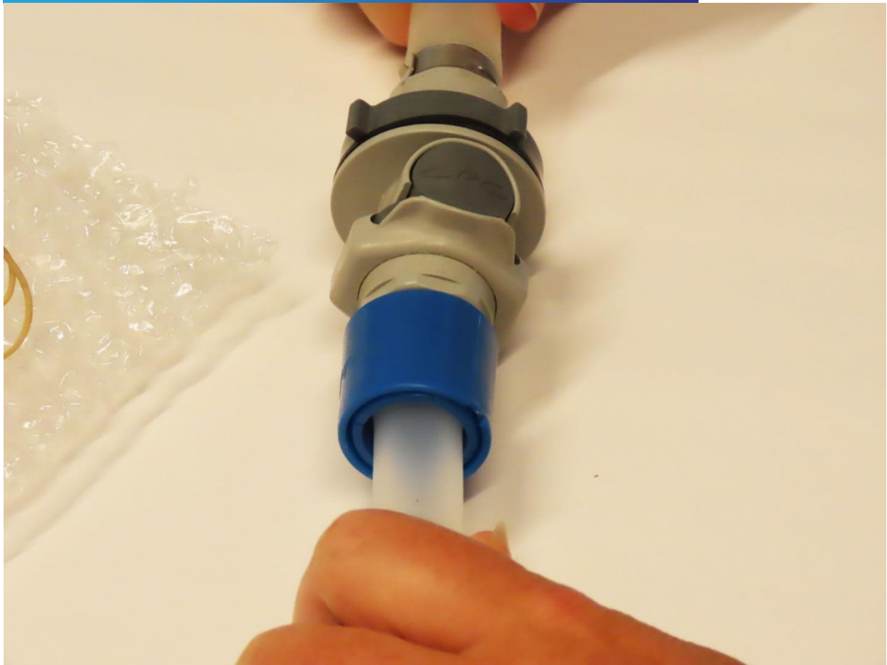
Figure 18. Process connector fully inserted into bag connector.
