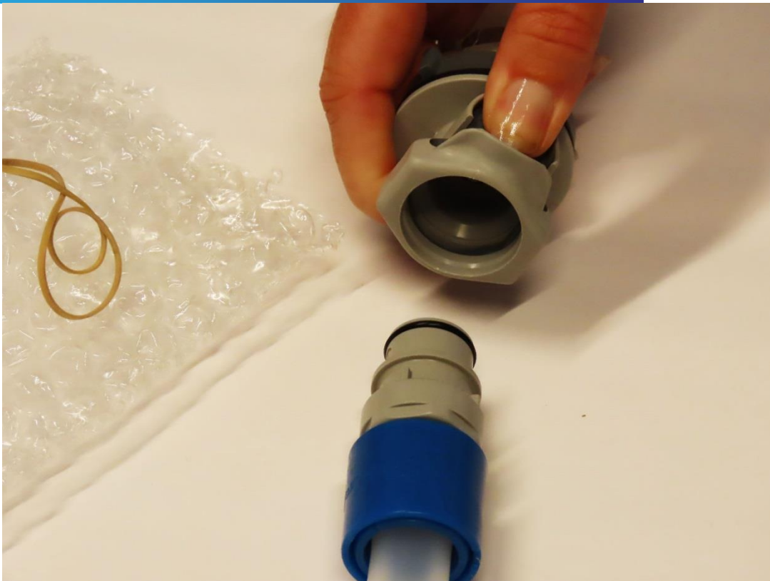
Figure 16. Preparing the bag connector to receive the process connector.
