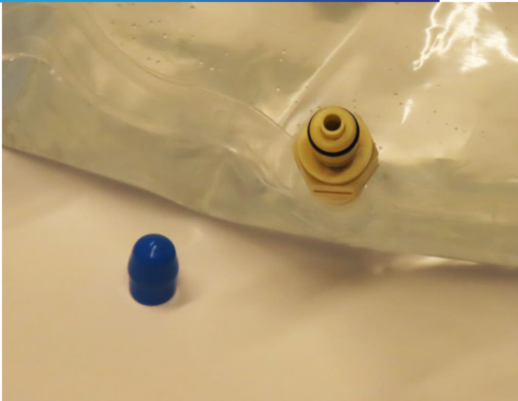
Figure 4. Bag with blue cap removed from fitment.
